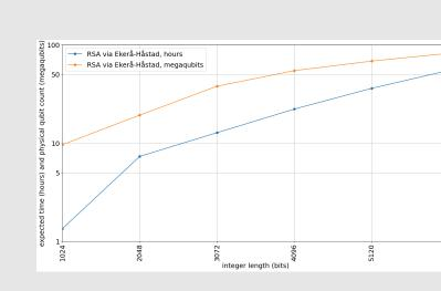
The time and qubit requirements for a quantum computer to factor integers of various lengths. 2048-bit integers, which many modern encryptions use, could be broken by a quantum computer with 20 Mqubits (20 million qubits) in about 7 hours.
